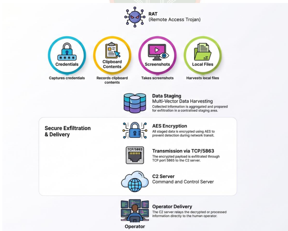
Figure: RAT Data Collection and Exfiltration (The Path of Stolen Data)
